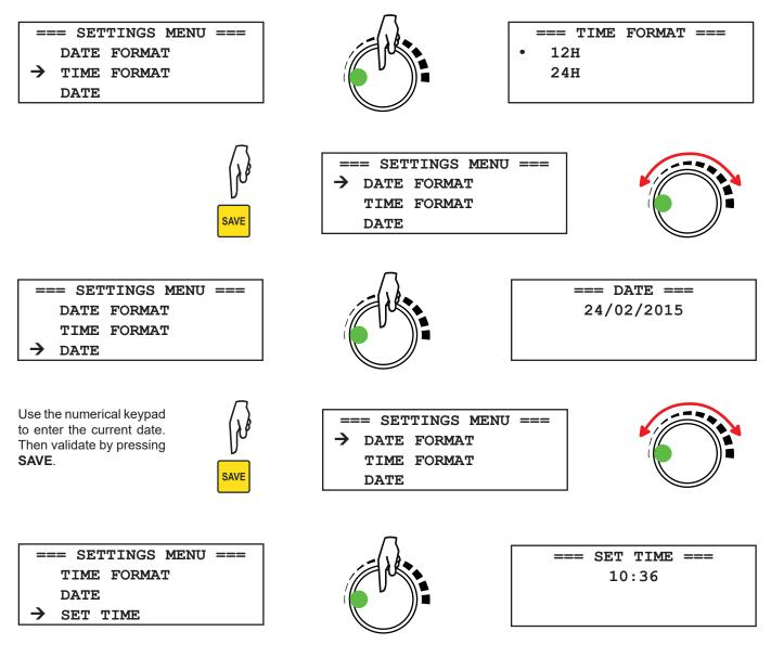
Use the numerical keypad to enter the time. Then validate by pressing the knob.
