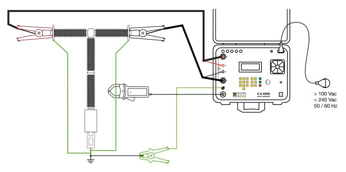
Tighten the terminals well to reduce the contact resistances and limit heating. Make sure that the leads are correctly uncoiled and do no form loops.
