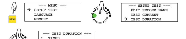
If you choose **TIMED**, program a test duration between 5 and 120 seconds using either the numerical keypad or the knob.
