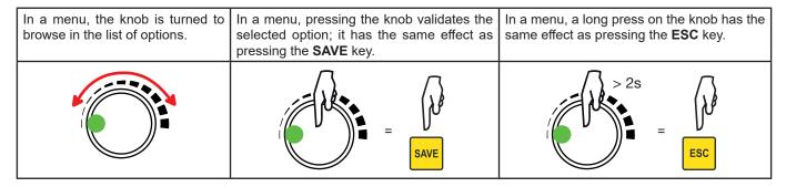
During a measurement in manual mode, it can be pressed to set the test current.
